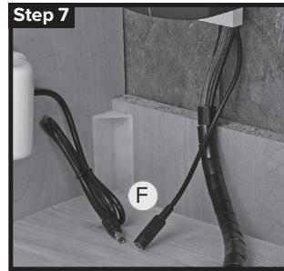
Connect the power connector to the battery box (F), install the refill and wait for a green light to flash on the E-cab. (See Refill Cartridge Loading for more detail.)
