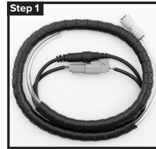
A 3 ft wire extension is available to add length between the Pump Pod and Refill Cabinet. The wire connections only fit one way. The tubing connector may need to switch sides based on which side is disconnected from the Pump Pod. Ensure all six lines are securely connected.
