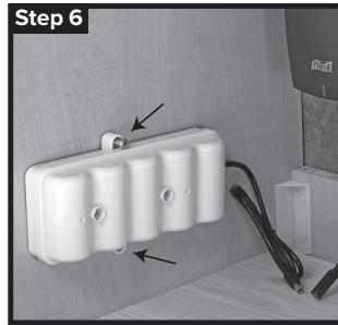
Position the battery box on a convenient (vertical or horizontal) surface under the countertop. Attach to the surface using the exposed holes to the sides of the box and two screws and anchors (if attaching to plaster or masonry surface).
