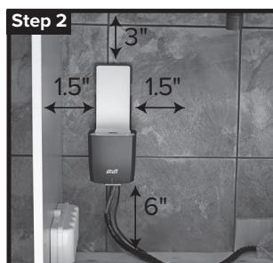
Install dispenser with at least 3" of free space above the cabinet, 1.5" on either side, and 6" below the closed cabinet to ensure functionality.
